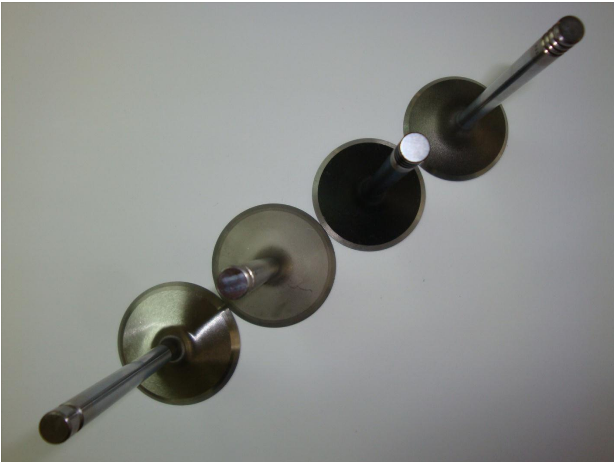
The exhaust valve we choose is 1.650 which is slightly bigger than stock, but it is bigger. You can see the valve size differences in the photo.
